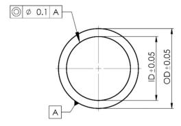
PT piezo tube actuators, dimensions in mm. Length L, outer diameter OD, and inner diameter ID see data table.
