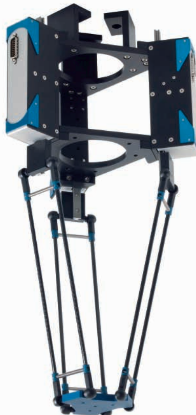
Pick-and-place systems are, for example, employed for automated drug pill filling equipment
