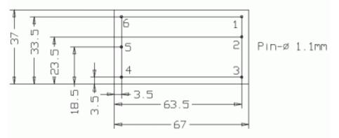
Figure 3: E-462.OE1, bottom view, dimensions in millimeters
