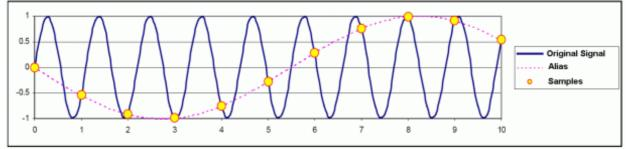
Fig. 11: Signal digitization with too low sample rate (time in 1/100 s): Original signal = 91 Hz and sampling rate = 100 Hz; the result is mistaked as a 9.1 Hz signal ("Alias")
