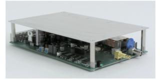
Fig. 2: E-617.00F high-power piezo amplifier OEM module
