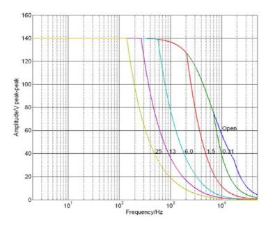
Fig. 6: E-617 open-loop frequency response with various PZT loads. Values shown are capacitance in  $\mu$ F.
